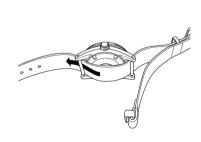
How to attach a pull-through type band
