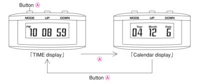
●When the display is changed, numerals and indications on the display screen scroll from right to left. Time display: Current time (hour, minutes, seconds)
