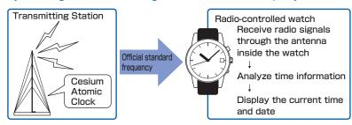
Time signal transmitted by a standard frequency is based on a super accurate "Cesium Atomic Clock" that may have a 1 second loss or gain per one hundred thousand years.
