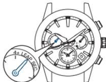
**When the leap second data reception is completed, the indicator hand returns to display the charging status. Use the watch as it is.**
