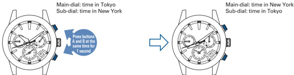
The second hand indicates the time zone for the basic time that was switched. The indicator hand indicates the setting status for DST (Daylight Saving Time) of the basic time that was switched. Afterward, the main-dial's hour and minute hands, sub-dial, date, and day switch, in that order. Finally, the second hand returns to the time display, and the indicator hand returns to the charging status display.
