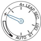
\* When the in-flight mode (X) is reset, the indicator hand indicates the charging status.
