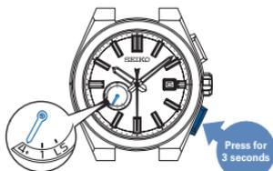
\* While the indicator hand points to "low" or "X", reception is not started even with operation for reception.
