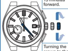
Turning the crown to the right moves the time 15 minutes forward.
