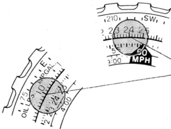
Find the position where the value on the dial ruler scale corresponding to 10 on the bezel ruler scale is the same as the value on the bezel ruler scale corresponding to 57.6 on the dial ruler scale.
