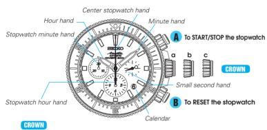
a) Normal position : winding up the mainspring (manual operation)
