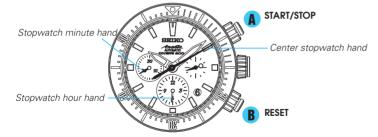
Current time indication: 10 o'clock 8 minutes and 42 seconds Stopwatch time indication: 6 hours 20 minutes and 10 seconds
