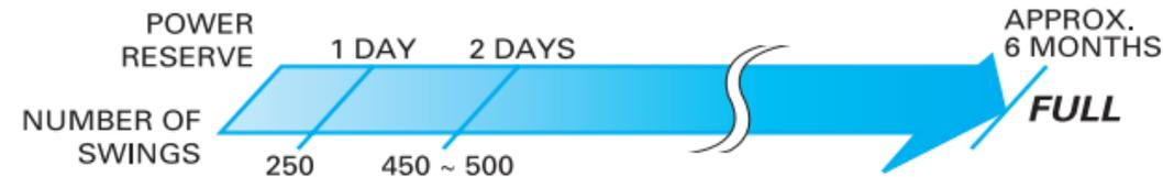
1. When the watch stops completely, or if you find the second hand moving at two-second intervals, swing the watch from side to side at a rate of twice a second.
