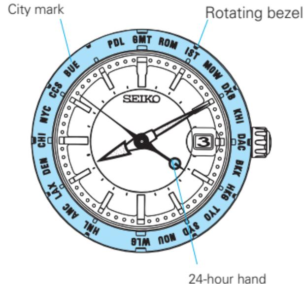
Turn the rotating bezel so that the city mark corresponding to the area whose time has been set in the "How to set the time" aligns with the 24-hour hand.
