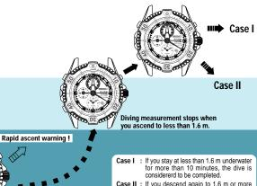
Case II: If you descend again to 1.6 m or more underwater before 10 minutes have elapsed, the two dives are considered inseparable, and the measurement is resumed.
