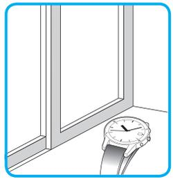
➤ After the second hand moves to the 0-second position and stops, the watch will start to receive radio signals.
