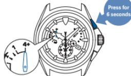
\* While the indicator hand points to "low" or ✈, reception is not started even with operation for reception.
