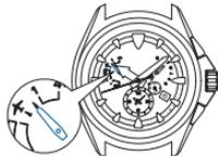
When the leap second data reception is completed, the indicator hand returns to display the charging status. Use the watch as it is.
