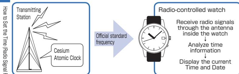
Time signal transmitted by a standard frequency is based on a super accurate "Cesium Atomic Clock" that may have a 1 second loss or gain per one hundred thousand years.
