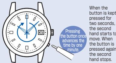
When the button is kept pressed for two seconds, the second hand starts to move. When the button is pressed again, the second hand stops.
