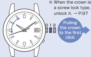
※ When the crown is pulled to the first click, the second hand advances 15 seconds and then moves back. Continue to conduct the operation.
