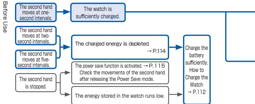
※ If the second hand does not move at one-second intervals even after fully charging the battery → "Charging the solar battery" in At Trouble on P.152
