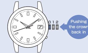
※ When the crown is a screw lock type, lock it. → P.97
