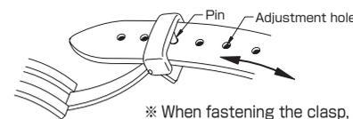
※ When fastening the clasp, insert the tip of the band into the movable loop and fixed loop, and then, securely tighten the clasp.
