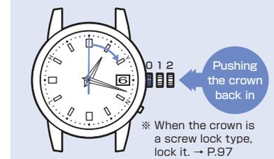
※ When the crown is a screw lock type, lock it. → P.97
