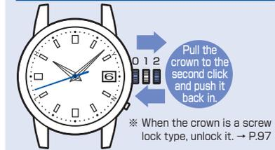
※ When the crown is a screw lock type, unlock it. → P.97
