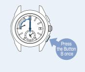
The watch automatically exits the preliminary position setting mode, and the second, hour and minute hands start moving.
