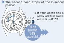
2 Keep pressing down the Button A and B at the Within 5 seconds after releasing the buttons, the second hand makes a full rotation and stops pointing to the 0-second position. Then the hour and minute hands will start to move and stop pointing to 12 o' clock 0 minutes. Button Press Simultaneously for 4 Seconds First, press the Button B, and subsequently press the Button A while
