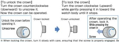
careful not to forcibly push it in, as doing so may damage the screw hole in the case 107
