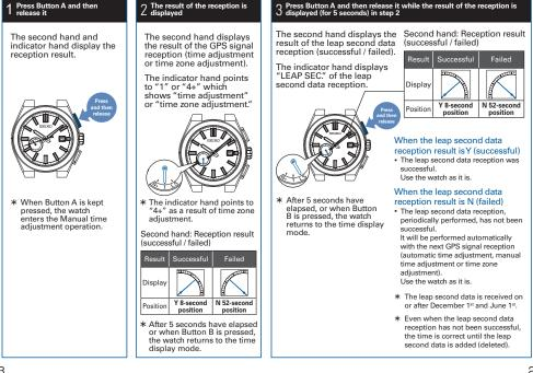
The results of GPS reception (time adjustment or time zone adjustment) and leap second data reception (successful /
