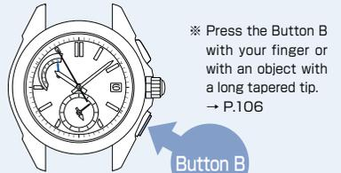
※ Press the Button B with your finger or with an object with a long tapered tip. → P.106
