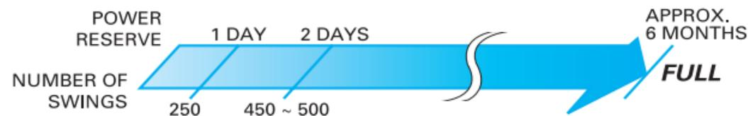
1. When the watch stops completely, or if you find the second hand moving at two-second intervals, swing the watch from side to side at a rate of twice a second.
