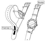
Pass the tip of the band through fixed loop 1 on the 6 o'clock side
