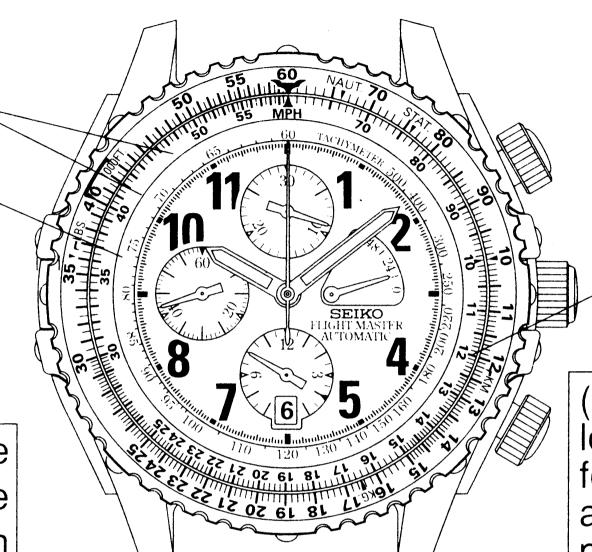
Logarithmic scale on rotary bezel
