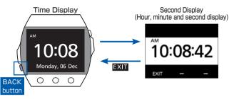
Press EXIT to return to the time display. If no button is pressed for approximately one minute, the watch automatically returns to the time display.
