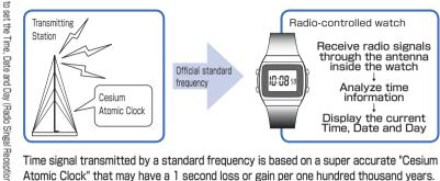
Time signal transmitted by a standard frequency is based on a super accurate "Cesium Atomic Clock" that may have a 1 second loss or gain per one hundred thousand years. 110
