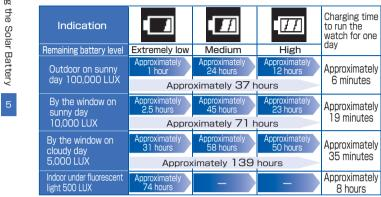
\* The time required to charge the watch may slightly vary depending on the model of the watch.
