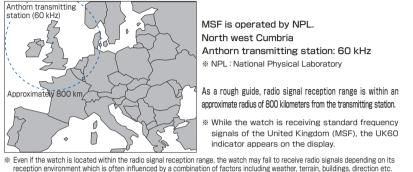
→ Conditions in which the watch may be unable to receive radio signals ⇒ P118
