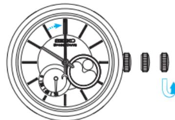
2. Turn the crown counterclockwise (the 6 o'clock direction) to set the minute hand slightly behind the time you wish to set, and then slowly advance it to the desired time.
