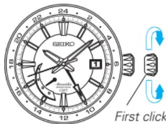
Clockwise: the hour hand turns counterclockwise. The date is set back one day when the hour hand makes two full rotations counterclockwise.
