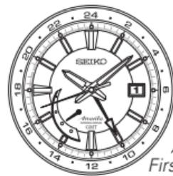
Clockwise: Setting the time back (The hour hand turns counterclockwise.)
