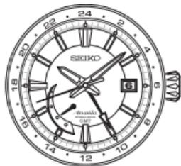
**<Mode 2>** Using the 24-hour hand to indicate the time in a different time zone.
