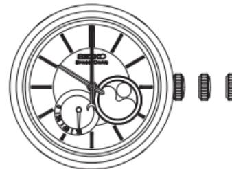
1. Pull out the crown to the second click when the second hand is at the 12 o'clock (0 second) position. The second hand will stop on the spot.
