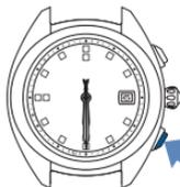
\* If the energy level is "low", reception will not begin even if GPS signal reception is operated. Expose the watch to light to charge it.
