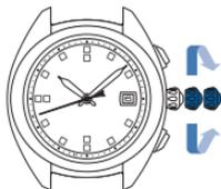
Turning the crown to the right moves the time forward.
