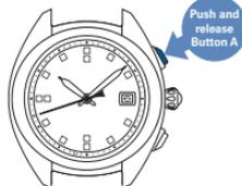
\* When Button A is kept pressed, the watch enters the Manual time adjustment operation.
