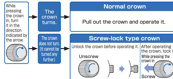
※ If your watch has a screw-lock type crown, the crown screws into the watch to prevent malfunction and increase water resistance.
