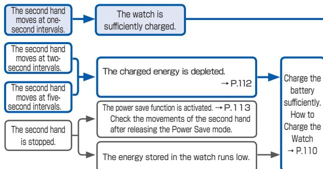
※ If the second hand does not move at one-second intervals even after fully charging the battery → "Charging the solar battery" in At Trouble on P.148
