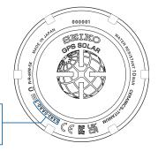
Caliber/case number The number to identify the watch type
