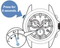
\* While the indicator hand points to "low" or ✈, reception is not started even with operation for reception.
