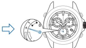
When the in-flight mode (λ) is set, the indicator hand does not indicate the charging status.
