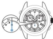
When the leap second data reception is completed, the indicator hand returns to display the charging status. Use the watch as it is.
