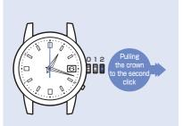
(5) Push the crown back in according to the time signal, etc.
